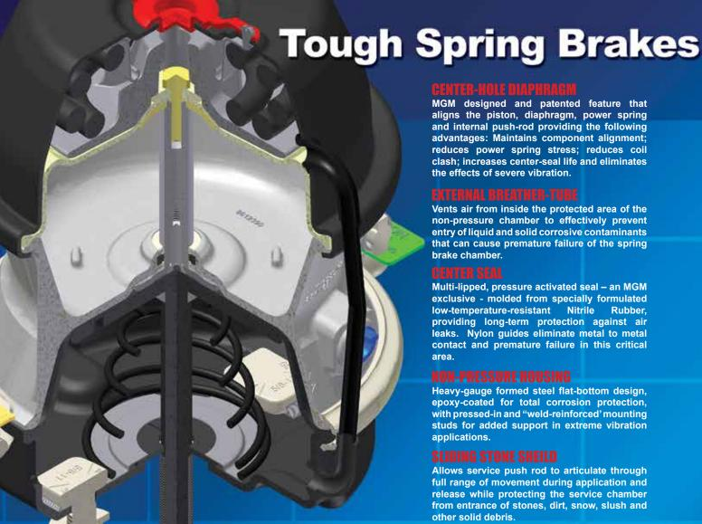
MGM designed and patented feature that aligns the piston, diaphragm, power spring and internal push-rod providing the following advantages: Maintains component alignment; reduces power spring stress; reduces coil clash; increases center-seal life and eliminates the effects of severe vibration.
