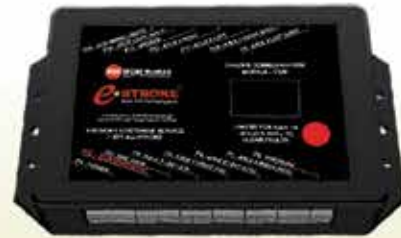
ECU - Electronic Control Unit
