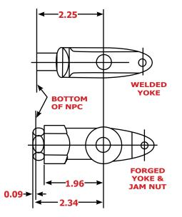
Units manufactured with a "welded" yoke have preset "Y" dimension, measured from the bottom of the NPC to the center-line of the yoke pin, of 2.25 - inches. Because the "Y" dimension is relatively short, the corresponding "X" dimension, measured from the bottom of the NPC to the end of the rod, will also be short, at approximately  $\frac{3}{4}$  of an inch.
