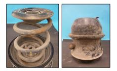
The MGM TR-TS (fully epoxy coated) breather tube brake pictured below is one of the preferred MGM brake models used in severe service and corrosive environments. The brake in the pictures below had been in service for one year showing how the breather tube has kept the interior of the spring brake preserved and in pristine condition.
