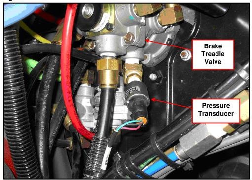
Figure 5: Pressure Transducer Mounted to Brake Treadle Valve
