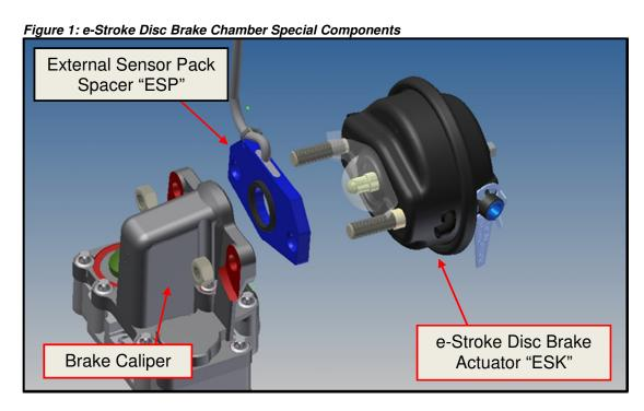
1.1.5: It is important to properly orientate the e-Stroke disc brake actuators. Mount the brake chamber so the sensor harness is orientated away from the brake rotor. Be aware that there are right and left hand actuators. See Figure 2.
