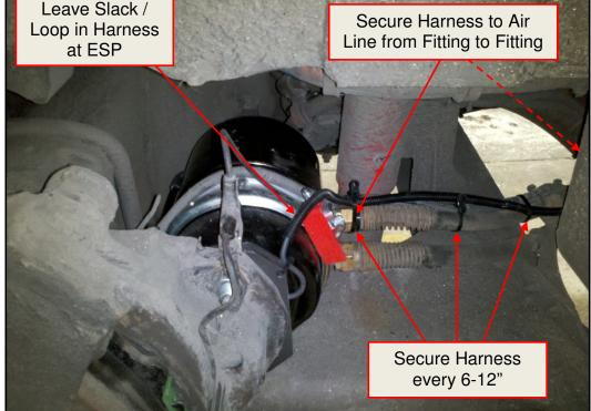
1.1.9: Reference EB 13-001 for additional Actuator, Sensor & Harness installation information.
