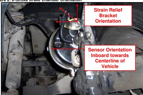
Figure 2: e-Stroke Brake Chamber Orientation
