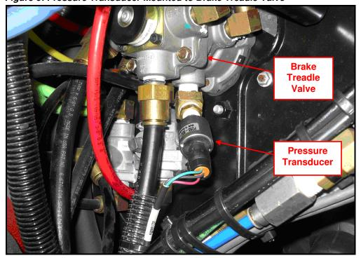
Figure 6: Pressure Transducer Mounted to Brake Treadle Valve
