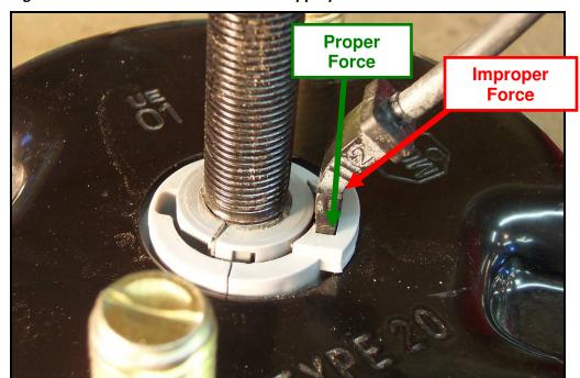
Figure 3: e-Stroke Sensor Installation – Appropriate Force Direction
