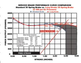
expansion. Lengthening the brake actuator's available stroke provides added "reserve" which increases the margin of safety. Long stroke actuators significantly improve braking performance during high demand braking and emergency situations.
