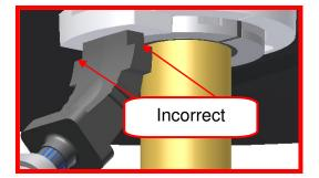
A stainless steel strain relief bracket is provided with the actuator to provide a means for securing the sensor pigtail to the vehicle to prevent the sensor from being inadvertently pulled out of the stone guard sensor port during normal vehicle operation. The strain relief bracket should be installed on the upper mounting stud of the actuator facing toward the centerline of the vehicle.
