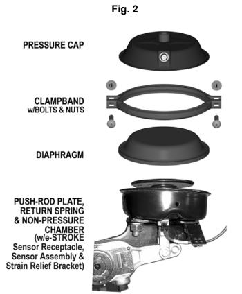
around the circumference of the clampband, release air from the chamber, loosen clampband nuts, then firmly tap around the circumference with a plastic hammer or rubber mallet while alternately tightening the clampband nuts in 5-10 Lbs.-Ft. increments to 30-35 Lbs.-Ft. of torque. Reapply air and check again.
