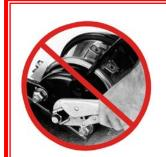
WARNING: DO NOT use vise-grip pliers to grip and lock the pushrod in place. This may damage the e-STROKE components and void your unit's warranty.
