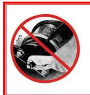
WARNING: DO NOT use vise-grip pliers to grip and lock the push-rod in place. This may damage the e-STROKE components and void your unit's warranty.
