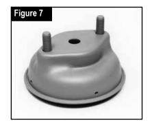
Apply air pressure to the service port of the brake until the service push-rod is fully extended and then measure and record both of the following dimensions outward from bottom face of service brake chamber (Figure 5):
