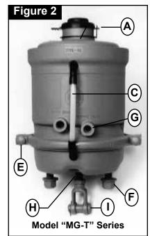
**IMPORTANT** - Unlike double diaphragm spring brakes, the unscrewing or removal of the release bolt does not cage the power spring, but only removes the power spring force from the slack adjuster. When an "MB" or "MB-T" model is manually released, the push-rod will extend in the "brakes applied" direction approximately 1/2-inch to 3/4-inch. The "MG-T" model will fully retract to the zero stroke position.
