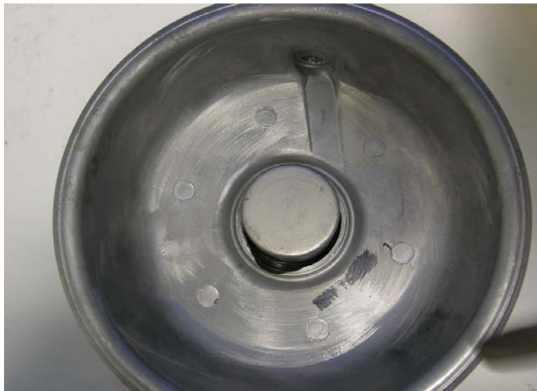
Leak @ Pushrod Seal (Photo 1)
