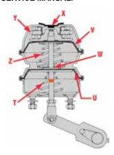
If air applied to the spring chamber has a tendency to apply the service brake, or to cause the service exhaust valve to leak, the push rod seal is leaking (W). (To verify, remove the service air line and apply air to the parking chamber. If air is detected coming through the open service air port, the push-rod seal is leaking.) Replace the entire piggyback as instructed in the appropriate MGM Brakes Service Manual.
