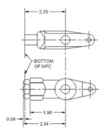
Determining the proper length to cut the rod is usually based on the rod length of the chamber being removed. A broken spring that prevents a spring-brake parking chamber from being fully caged sets the stage for cutting the rod too short, altering the geometry of the brake linkage.
