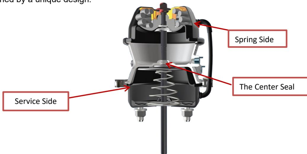
The modern spring brake actuators design consist of two main sections, the parking spring chamber, which houses the power spring providing the functions for parking and for emergency brake actuation, and the service chamber, which provides the function to stop the vehicle during normal road operation. These two sections work as a unit to comprise the total function of the spring brake actuator.
