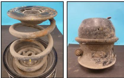
The MGM TR-TS (fully epoxy coated) breather tube brake pictured below is one of the preferred MGM brake models used in severe service and corrosive environments. The brake in the pictures below had been in service for one year showing how the breather tube has kept the interior of the spring brake preserved and in pristine condition.
