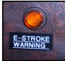
Tractor CCM turns on dash warning light for Tractor or Trailer brake fault
