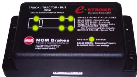
e-Stroke tractor and trailer systems are designed to operate both independently and together. An e-Stroke tractor system will display the tractor brake conditions on the tractor CCM. In addition an optional dash warning light may be installed on the dash of the vehicle, which will illuminate with an active brake fault on the tractor and up to three trailers.
