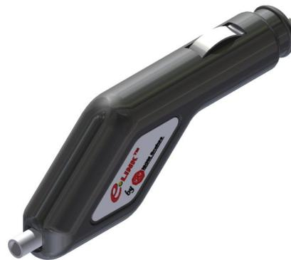
If the e.LINK LED remains off, this indicates no communication is present between the e.LINK device and the Trailer CCM or a Tractor e-Stroke System is present. The e.LINK device is designed to work only when a Tractor e-Stroke System is not present on the Tractor.
