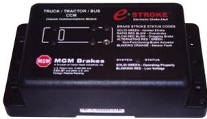
After the vehicle ignition has been activated, the CCM will enter start-up mode. During this time, the software version will be indicated via a blink code on the System Status LED. Until, the CCM has completed the self diagnostic test, all actuator specific LEDs will remain blank.
