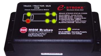
Concurrently, the warning device driver will energize the external warning device (if installed) and the appropriate SAE J1587 fault message will be broadcast on the SAE J1708 bus. Once, the fault condition is no longer true, the wheel specific LED will revert back to solid green, the warning device will de-energize, and the SAE J1587 fault code will be broadcast as inactive.
