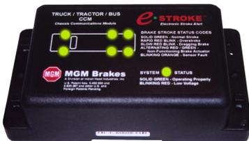
The Chassis Communication Module (CCM) is the “brains” of the e-STROKE system. The CCM provides regulated power to the actuator sensors and the pressure transducer. The actuator sensor and pressure transducer inputs are continuously monitored by the CCM to determine whether the stroke of each of the actuators is in proportion to the air pressure applied by the brake system.
