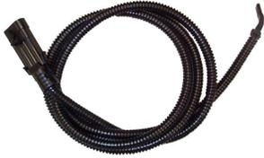
The e-STROKE sensor is a non-serviceable, replaceable component constructed with an over-molded sensor device and the connection pigtail. Care must be taken during installation to insert the sensor into the stone guard sensor port with the proper alignment. The sensor end must be inserted perpendicular to the face of the stone guard until the sensor is completely seated.
